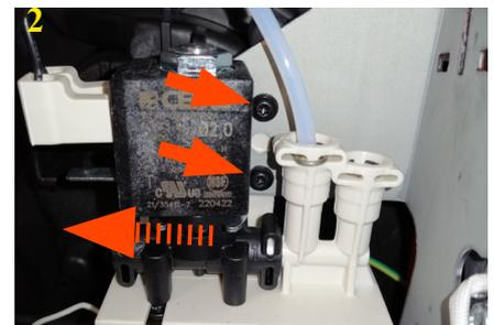
2 Unscrew the screw shown and lift 2way valve
