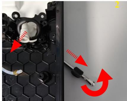
2 Unscrew the steam sprayer, lift the tube handgrip and the steam tube
