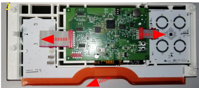
3 Lift the led cover, disconnect the cables and turn the principal CPU
