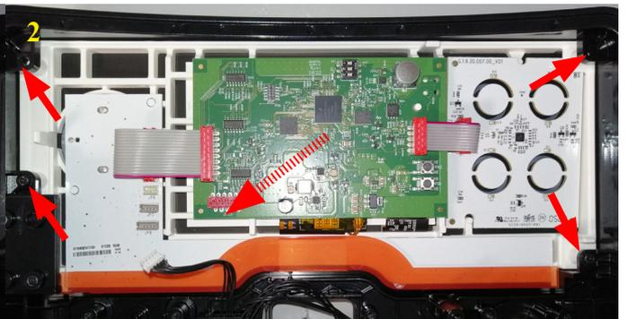
2 Unscrew the screw shown and lift the UI assy
