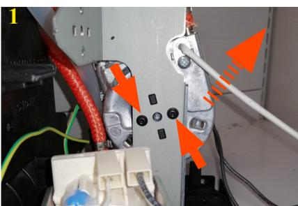
1 Unscrew the screw shown and lift the boiler
