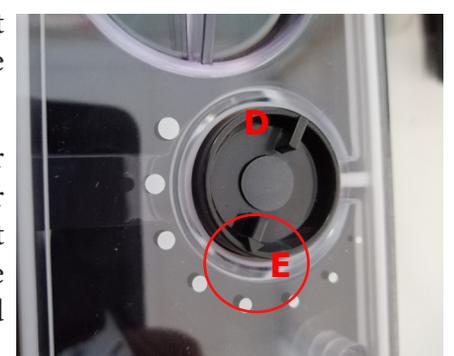
If there are coffee powder residues between the two grinding blades it is recommended to tighten by max. two brands at a time.
