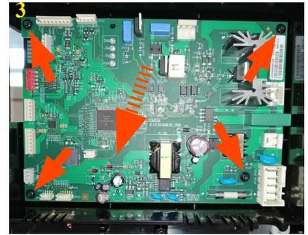
3 Unscrew the screw shown and lift Main board
