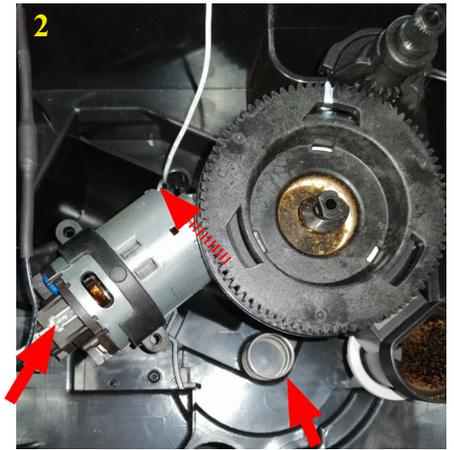
2. Lift the coffee grinder and disconnect the electrical wiring. When reassembling the coffee grinder, make sure the spring is repositioned correctly.
