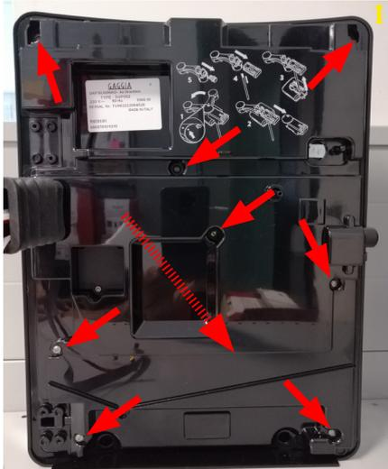
1 Unscrew the screw shown and lift the cover panel
