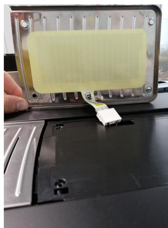
Unscrew the screw shown if you want replace the haet element+cover casing of cup warm (pos 108 of exploded view)
